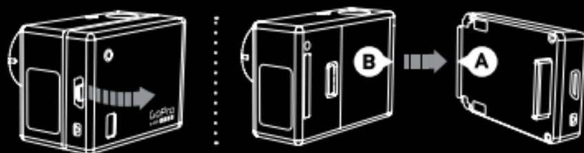
1. Pull back on the left side of the Battery BacPac marked with arrow to disconnect from the HERO Port.
