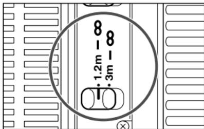
You can set the focusing distance range to 1.2 m/3.9 ft. to infinity or 3 m/9.8 ft. to infinity. By setting the suitable focusing distance range, the actual autofocus time can be shorter.
