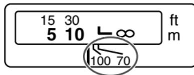
The infrared index corrects the focus setting when using monochrome infrared film. Focus on the subject manually, then adjust the distance setting by moving the focusing ring to the corresponding infrared index mark.
