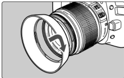
Turn the hood in the direction of the arrow to attach it securely.
