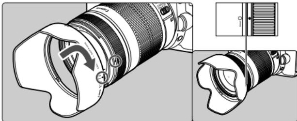
The EW-73B hood can keep unwanted light out of the lens, and also protects the lens from rain, snow, and dust.
