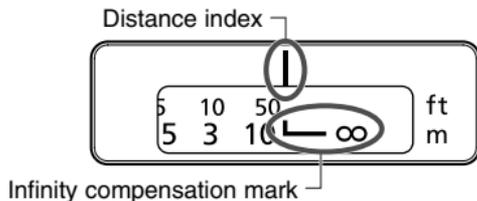
To compensate for shifting of the infinity focus point that results from changes in temperature. The infinity position at normal temperature is the point at which the vertical line of the L mark is aligned with the distance indicator on the distance scale.
