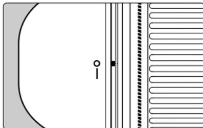
To attach the hood, align the hood's attachment position mark with the red dot on the front of the lens, then turn the hood as shown by the arrow until the lens' red dot is aligned with the hood's stop position mark.
