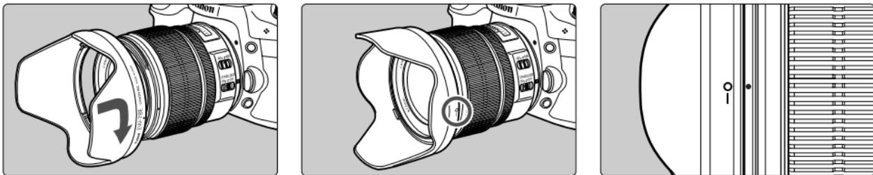
To attach the hood, align the hood's attachment position mark with the red dot on the front of the lens, then turn the hood as shown by the arrow until the lens' red dot is aligned with the hood's stop position mark.
